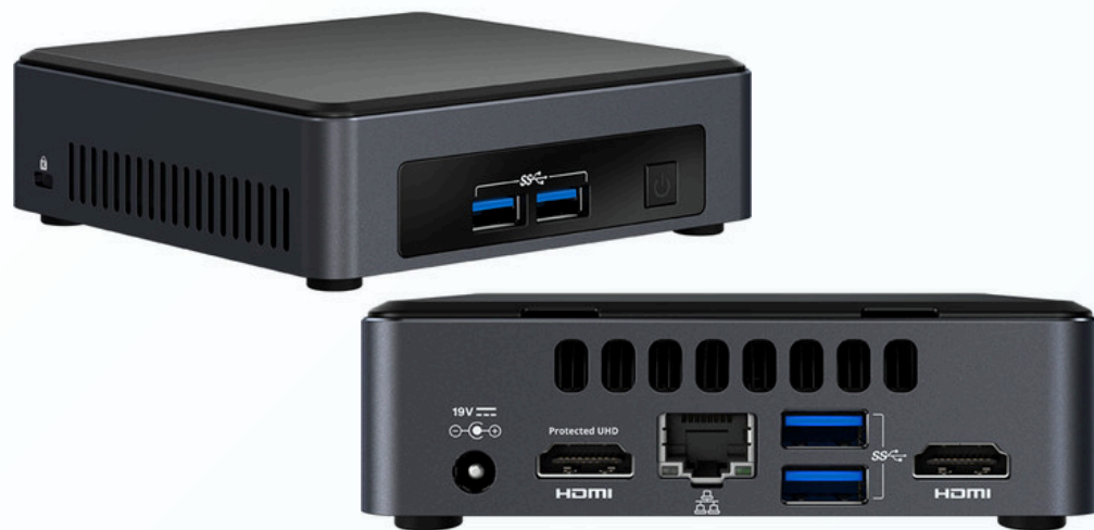
The actual servers (not staff terminals), palm-sized: 117 × 112 × 36 mm
